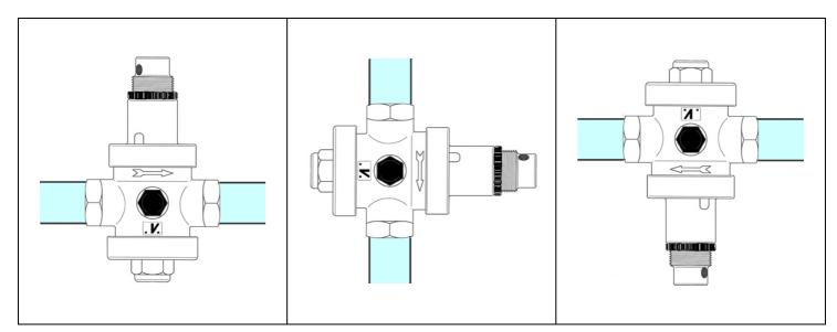
Pressure reducing valves can be damaged by dirty water; therefore we advise to install a self-cleaning filter upstream before the pressure reducer, in order to protect the valve and any other mechanism (thermostatic mixers, taps, etc.).
